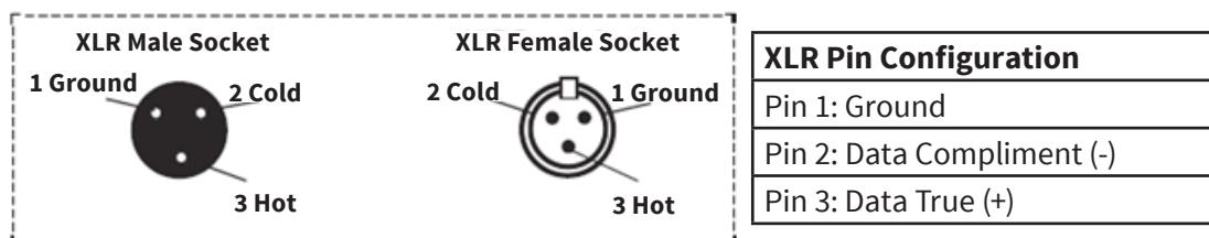
**Special Note:** Line Termination. When longer runs of cable are used, you may need to use a terminator on the last unit to avoid erratic behavior. A terminator is a 110-120 ohm 1/4 watt resistor which is connected between pins 2 and 3 of a male XLR connector (DATA + and DATA -). This unit is inserted in the female XLR connector of the last unit in your daisy chain to terminate the line. Using a cable terminator will decrease the possibilities of erratic behavior.
